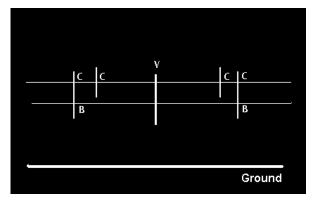
NOTE The visual aim procedure for US DOT headlamps marked VOR or VO does not require the lower horizontal line. Simply connect your +C marks with a horizontal line.
