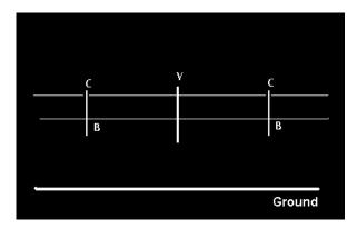
Or like this for a system of two low- or low/high beam plus two high-beam lamps:
