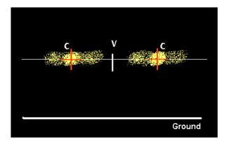
Make sure to work on one lamp at a time. It is best to disconnect the power to the headlamp you are not working on, so light from the other lamp's beam pattern doesn't mislead your eyes. Also be sure to disconnect or cover the adjacent high/low beam lamp when you are aiming its high-beam-only neighbour.
